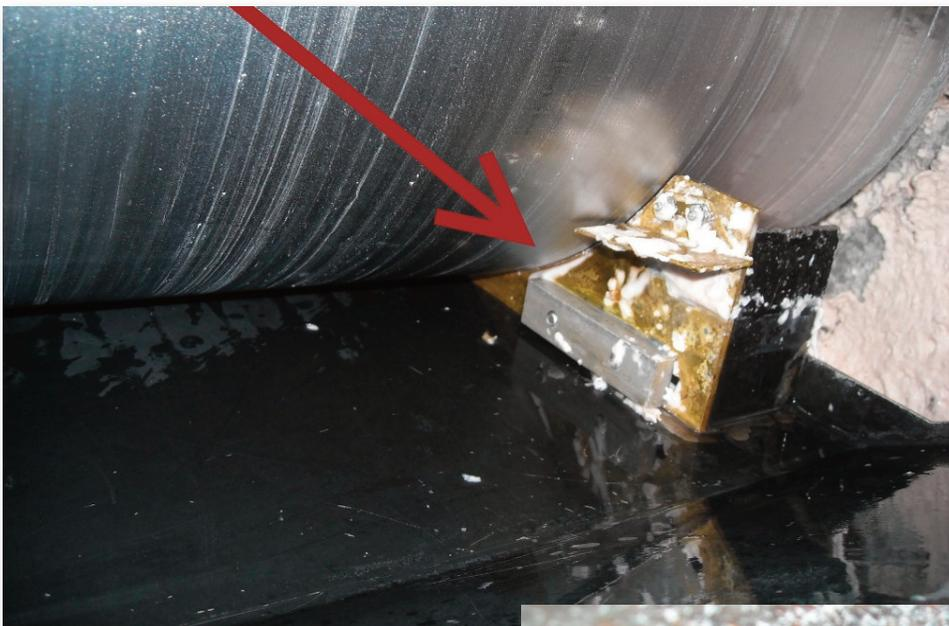
condition to properly seal the edge to hold a solid pattern. This brass dam must be loosened and pushed against the roll regularly to compensate for wear. The picture below illustrates a properly set brass dam and wiper.
