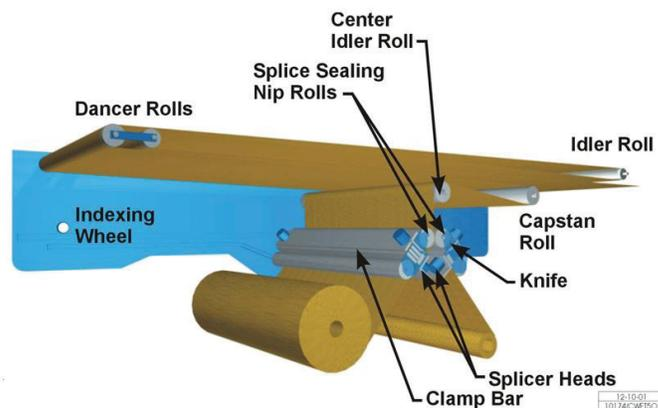
the splicer creating a surplus of paper to draw on during the splice sequence. During the splice, the dancer roll moves toward the primary idle roll, allowing the corrugator to pull from this reserve of paper. This allows time for the new roll being spliced to slowly start unwinding and increase in speed so less force is exerted on the splice joint. After the splice is made, the dancer roll automatically moves back into the home
