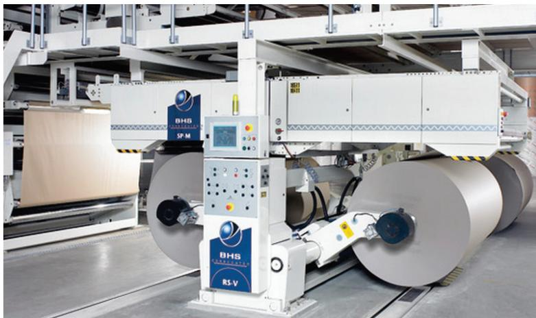
It is estimated that automatic splicers should operate at a success rate of 98% or above to minimize the costs associated with waste and downtime. The time lost because of poor splicing can be calculated by multiplying the splicer efficiency by the number of splices in a year
