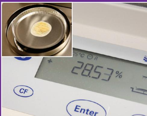
An infrared (IR) moisture meter, common in box plants to check paper and combined board moisture, can also be used. Just set a weigh dish in the meter and zero the scale, add 3 grams to 5 grams of adhesive, close the lid and run the test. This type of meter takes only 8 minutes to 12 minutes to run.
