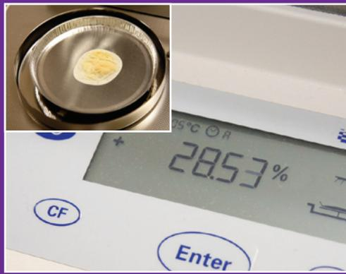
*An infrared (IR) moisture meter, common in box plants to check paper and combined board moisture, can also be used. Just set a weigh dish in the meter and zero the scale, add 3 to 5 grams of adhesive, close the lid and run the test. This type of meter takes only 8 to 12 minutes to run.*
