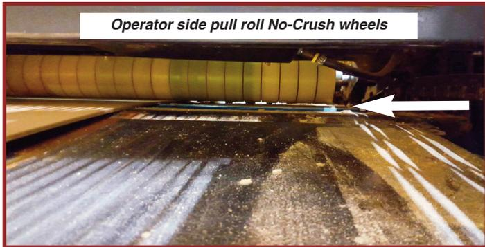
**Replacement.** The service life of No-Crush wheels can vary and will depend on the amount of board produced. Their physical appearance will give you the best indication when they need to be replaced. If any of the spokes are broken or if the spokes become visible on the outer diameter of the wheel (there will be small depressions between each spoke) the wheel should be replaced. Periodic visual inspections are the best way to monitor the condition of No-Crush wheels.
