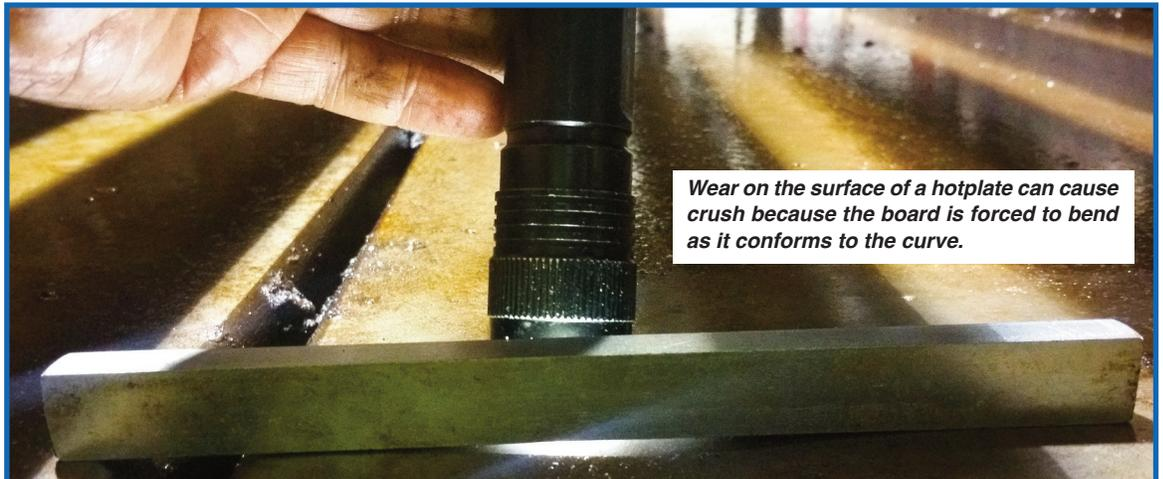
*Wear on the surface of a hotplate can cause crush because the board is forced to bend as it conforms to the curve.*
