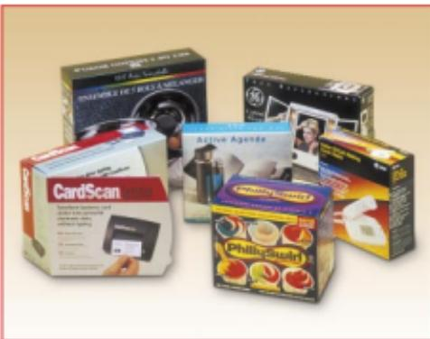
Litho liners cold-bonded to miniflute single face produce an attractive and economical alternative to folding carton packaging. (Package samples courtesy Accurate Box Company, Inc., Paterson, New Jersey.)
