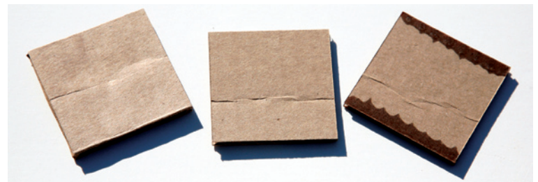
The failure of ECT samples is often accompanied by interflute buckling (above, left). This defect is similar to the patterned buckling of the liner board facings, which occurs during the compression test.
