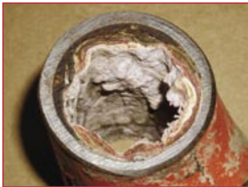
Liquid starch adhesive not only bonds the paper together, it also bonds itself—and any chemicals in it—to the inside of the distribution system's pipes.
