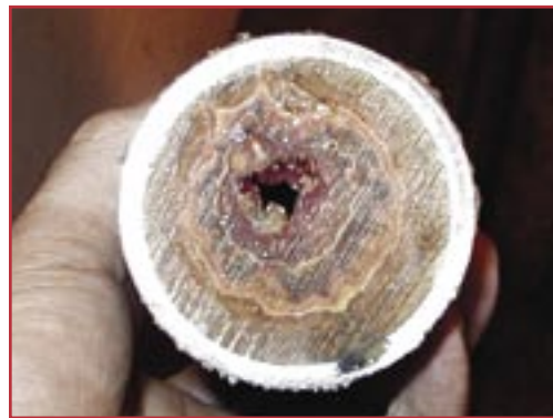
Liquid starch adhesive not only bonds the paper together, it also bonds itself—and any chemicals in it—to the inside of the distribution system's pipes.
