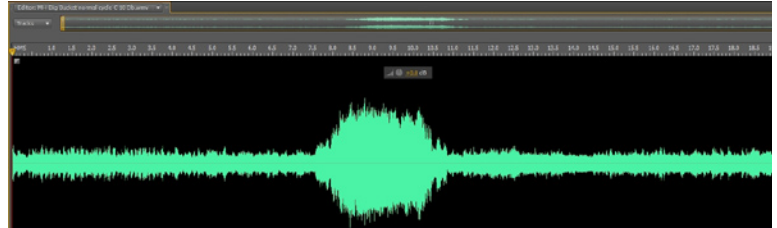
Graph of a bucket trap. Note the marked change in the middle of the graph when the trap cycles.
