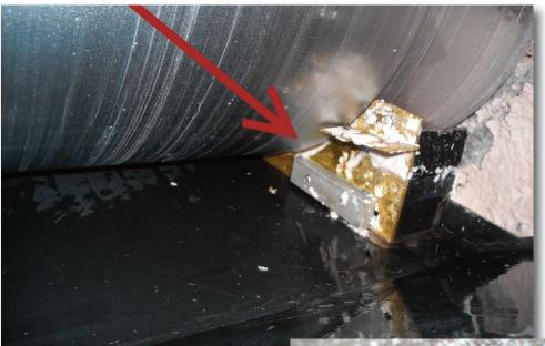
condition to properly seal the edge to hold a solid pattern. This brass dam must be loosened and pushed against the roll regularly to compensate for wear. The picture below illustrates a properly set brass dam and wiper.
