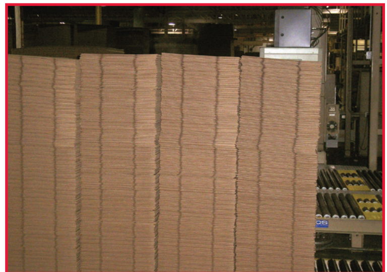
Uneven stacking is evidence of a board crush problem.
