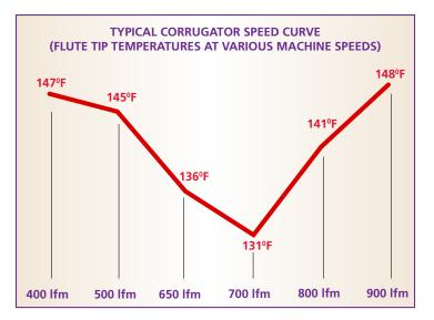
(as does bond quality). This is because, at very high speeds, the web spends very little time on the bridge, losing very little of its heat energy, therefore needing very little time on the preheater to replace lost energy. The accompanying graph demonstrates this phenomenon.
