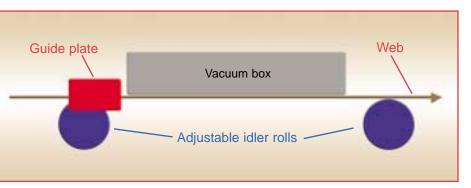
during width changes. When the double backer operator reduces or turns off the vacuum the web immediately moves to one side and contacts the guide plate. When the operator opens the side guides for the next paper width, the paper continues to walk off center, requiring corrective action.
