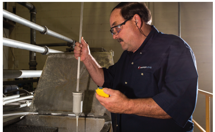
Checking viscosity using a Love Cup
