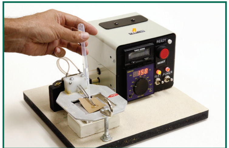
Our laboratory uses an electronic timer to measure penetration of liquids through various substrates.
