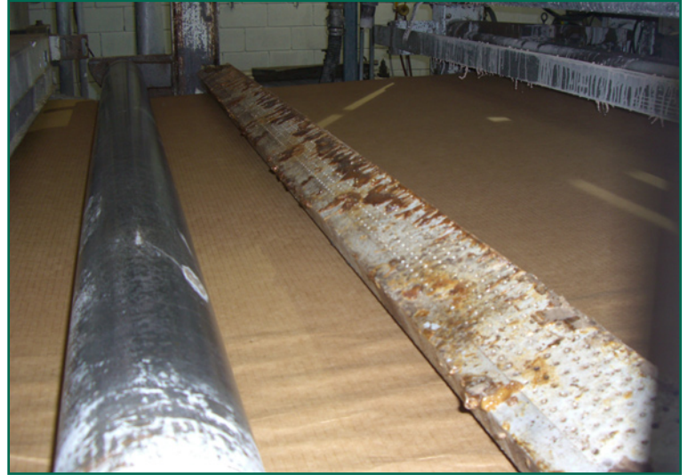
The location of the Jet Assist manifold on the corrugator makes it vulnerable to dust, adhesive, and debris. Regular maintenance will prevent performance failure.
