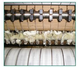
Finger-type machines were often troubled by low gel-temperature adhesives gelling on the fingers.
