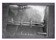
The secondary mixer (left) uses a set of marine type propellers to mix the cooked primary portion into the slurry. These tanks are usually rectangular in shape, with vee-shaped bottoms. A shaft runs horizontally across the bottom of the vee with
