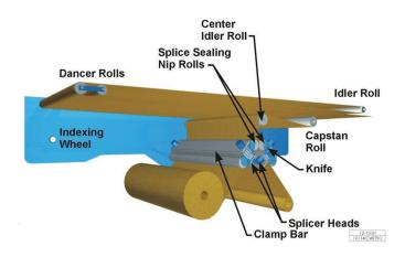
the splicer creating a surplus of paper to draw on during the splice sequence. During the splice, the
