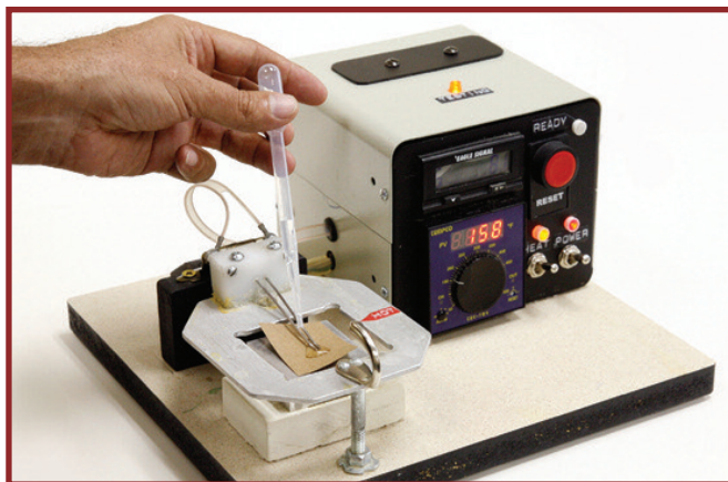
Our laboratory uses an electronic timer to measure penetration of liquids through various substrates.
