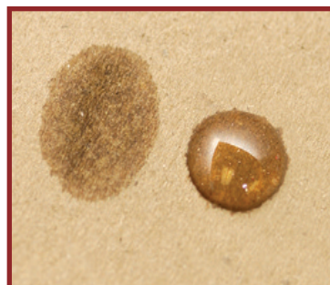
Plain water bead on right was applied first. At the time of the photograph, it had been sitting on the paper surface for several minutes. The spot on the left shows where water with XM-5 penetrant absorbed instantly.
