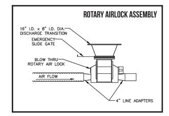
Once the stream of air current is established from the blower to the mixer and back to the silo, a rotary airlock on the bottom of the silo starts turning and the corn starch is metered into the air flow.
