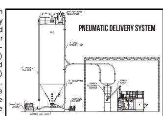
approximately 20' of the mixer. If this is not practical, the silo can be located where there is adequate room on the property, and starch is then delivered to the mixer by a pneumatic delivery system.
