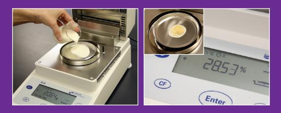
An infrared (IR) moisture meter, common in box plants to check paper and combined board moisture, can also be used. Just set a weigh dish in the meter and zero the scale, add 3 grams to 5 grams of adhesive, close the lid and run the test. This type of meter takes only 8 minutes to 12 minutes to run.
