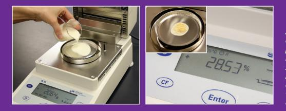
An infrared (IR) moisture meter, common in box plants to check paper and combined board moisture, can also be used. Just set a weigh dish in the meter and zero the scale, add 3 to 5 grams of adhesive, close the lid and run the test. This type of meter takes only 8 to 12 minutes to run.
