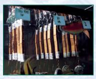
for produce and vegetable boxes that will need high resistance to water over a long period of time. The board sample is cut into 10 strips 3/4" x 6". A hole is punched in each end, one to hang the sample from and one to hang a 250g weight from. The sample
