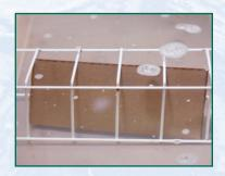
bond strength is tested with a comb like fixture inserted through the flutes in a crush tester. The results are reported in pounds of force per lineal foot of glue line tested (lbs/lin ft). Ideal test results are 1-2 lb/ft for WRA and 3-4 lb/ft for WPA.
